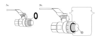
4. On the inside of the cooler, place the large 0-ring on the nipple and push it against the inside wall of the cooler.
