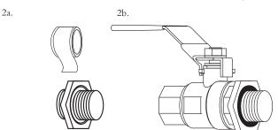
**3.** Place the small O-ring on the nipple and push it all the way into the groove of the locknut, then insert the assembly through the hole in the cooler.The O-ring should be resting on the outside of the cooler.
