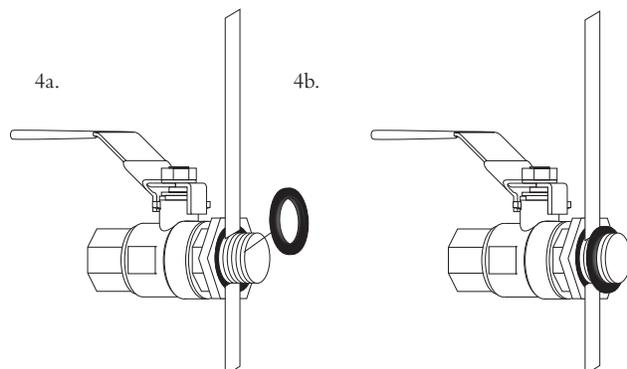
5. Slide the Washer(s) onto the nipple, then thread on the coupler. Hand tighten the coupler until snug, then tighten further by holding the coupler in place and rotating the valve until hand tight.
