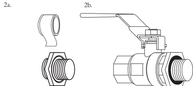
3. Place the small O-ring on the nipple and push it all the way into the groove of the locknut, then insert the assembly through the hole in the cooler. The O-rings should be resting on the outside of the cooler.
