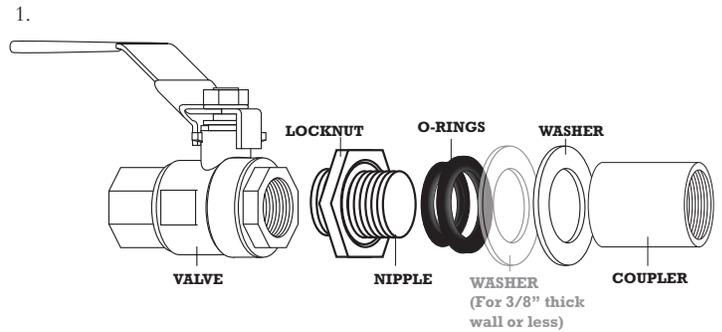
2. Ensure the locknut is threaded on to the nipple as far as it will go. Apply 3 wraps of thread tape to the nipple (on the side where fewer threads are showing), and then thread into the ball valve.
