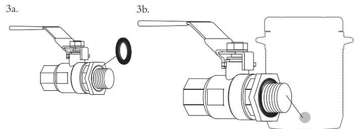
4. On the inside of the cooler, place the large O-ring on the nipple and push it against the inside wall of the cooler.
